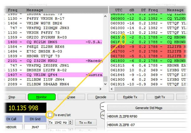
9.38 Keep an eye on the waterfall. If you notice FT8 signals shifted towards the left or right side, check that your rig's VFO frequency is correct for the band you're using.
