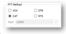
VOX, make sure the radio's VOX sensitivity is high enough to trigger reliably at the audio level you are using, and hold-in for the entire over.
